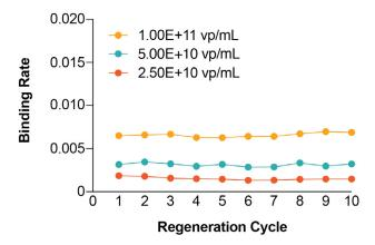
Performance up to 10 regenerations at 3 concentrations of the same probes with no observed loss in binding rate.
