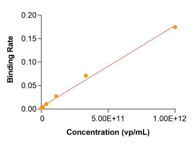
The graph shows an AAV9 standard curve for concentrations 3.00E+09 to 1.00E+12 (vp/mL). The binding rate between the analyte and the probe surface is a measure of the analyte concentration.
