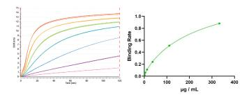
Binding curves and standard curve for PEGylated liposomes (1  $\mu$ g/mL to 300  $\mu$ g/mL in PBS + 0.2% BSA).
