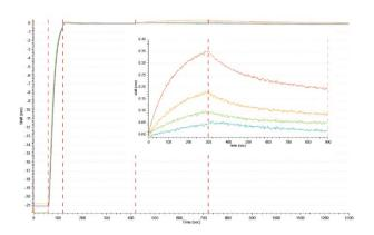
Binding between PEGylated LNP and Apo-E. LNP was loaded at 20  $\mu$ g/mL. Positive signal is observed for LNP loading and subsequent Apo-E association. Sensorgram shows association between 2.5, 5, 10 and 20 nM of Apo-E for 300 sec followed by dissociation for 900 sec.
