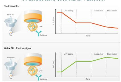
Gator's Anti-PEG probes allow analysis of PEGylated LNPs without the signal inversion observed in traditional BLI. This is due to innovative optical layer and novel surface chemistry.
