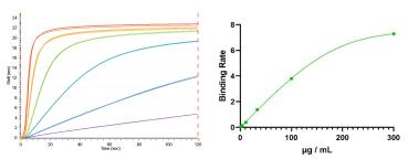
Binding curves and standard curve for PEGylated LNPs (1 µg/mL to 300 µg/mL in PBS+0.2% BSA).
