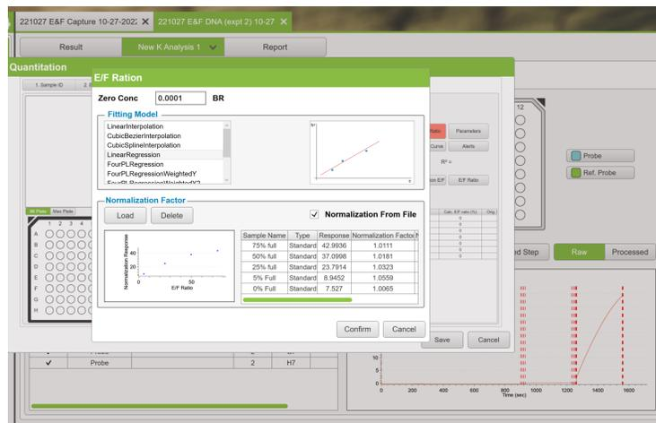
5. Click on "Cal. E/F Ratio". Ratio has been determined and file can be saved
