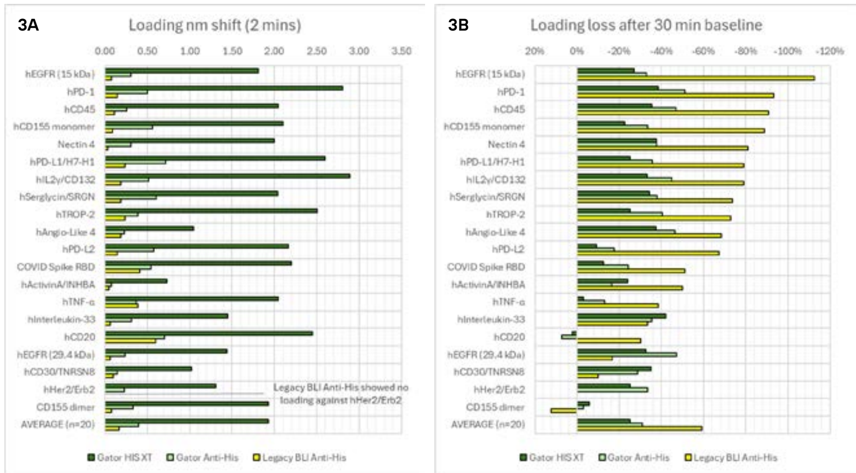
Figure 3. Ligand binding performance of Gator HIS XT, Gator Anti-His, and legacy BLI anti-His probes. 3A: Loading shift using 1 \mu g/mL of protein for 2 minutes. Values reported are final response. 3B: After loading experiment, loaded probes were placed in baseline buffer for 30 minutes. Total reduction in signal is reported as a percentage for ease of comparison.
